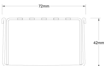
Grates longer than 1500mm supplied in sections. Tile Inserts longer than 1200mm supplied in sections. Channels over 3000mm supplied in sections with joiner. +/-2mm tolerance on dimensions.
