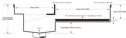
Grates longer than 1500mm supplied in sections. Tile Inserts longer than 1200mm supplied in sections. Channels over 3000mm supplied in sections with joiner. +/-2mm tolerance on dimensions.
