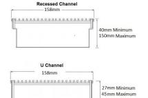
Grates longer than 1500mm supplied in sections. Tile Inserts longer than 1200mm supplied in sections. Channels over 3000mm supplied in sections with joiner. +/-2mm tolerance on dimensions.
