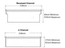
Grates longer than 1500mm supplied in sections. Tile Inserts longer than 1200mm supplied in sections. Channels over 3000mm supplied in sections with joiner. +/-2mm tolerance on dimensions.
