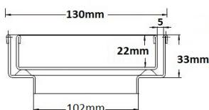
Grates longer than 1500mm supplied in sections. Tile Inserts longer than 1200mm supplied in sections. Channels over 3000mm supplied in sections with joiner. +/-2mm tolerance on dimensions.
