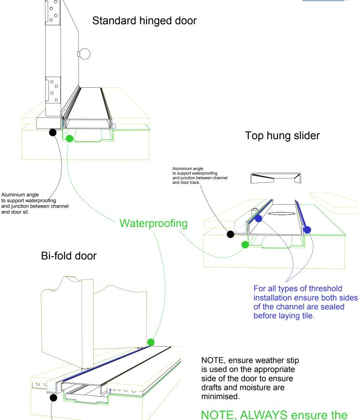
Aluminium angle to support waterproofing and junction between channel
