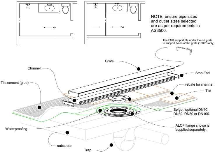
NOTE, this method requires the channel system to be ABOVE and SEPARATE from the WATERPROOFING.
