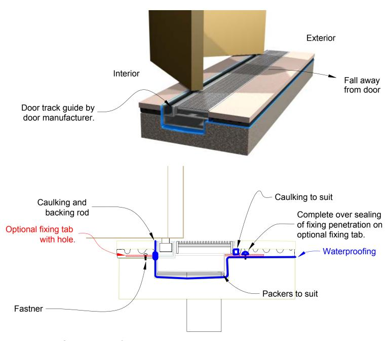
Outlet size and frequency is determined by a hydraulic consultant. Standard outlet sizes are DN50, 80 & 100. Install as per waterproofing AS3740.
