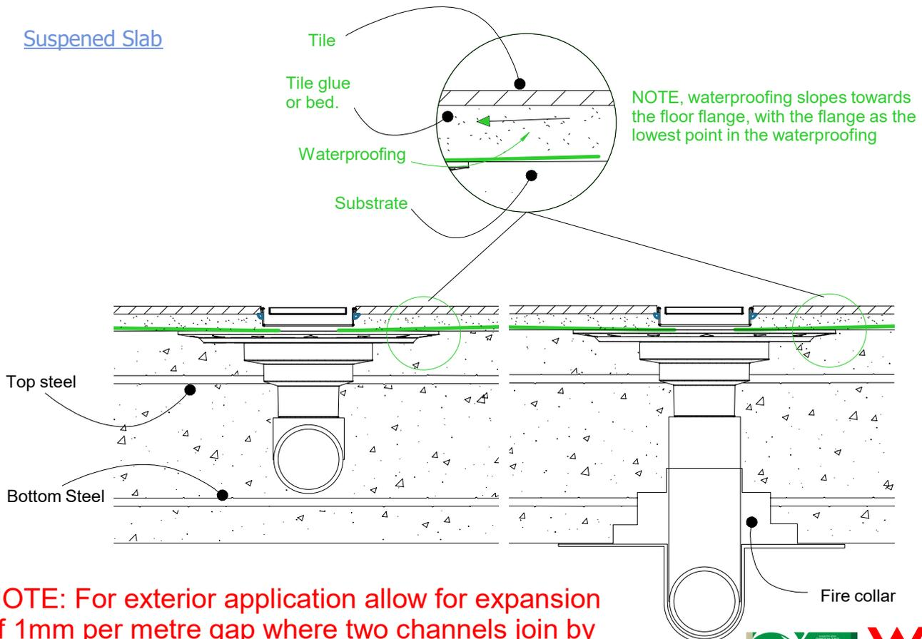
**NOTE: For exterior application allow for expansion of 1mm per metre gap where two channels join by using quality suitable flexible sealant on channel joiners.**
