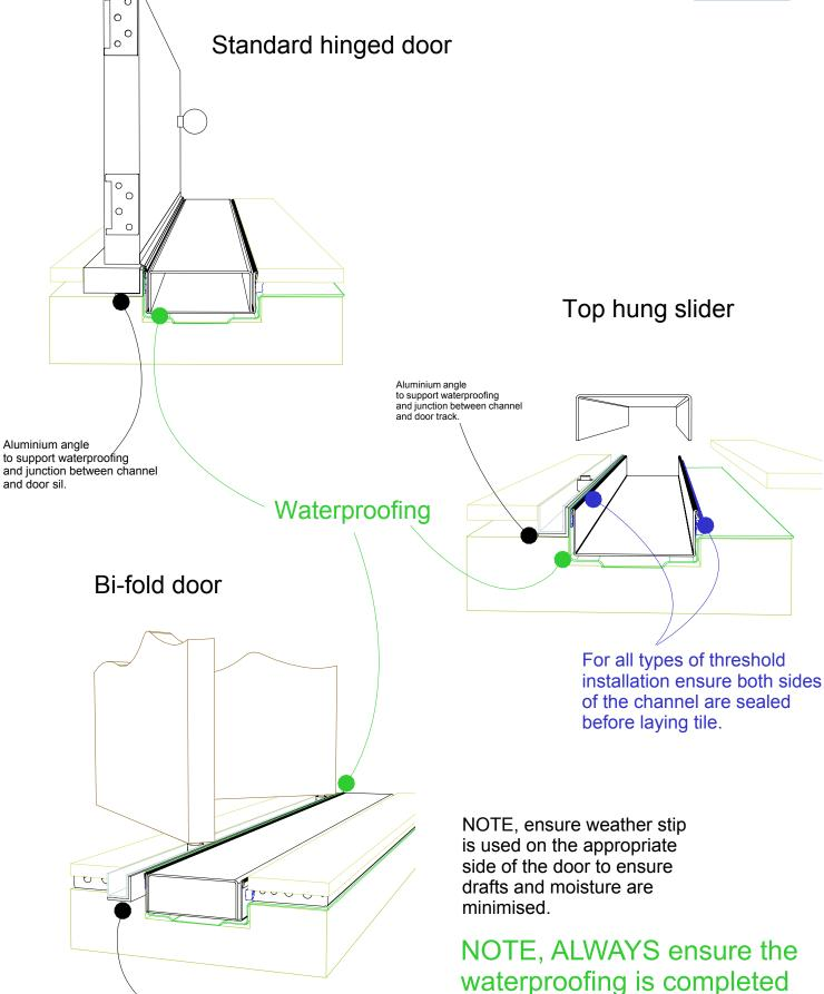
Aluminium angle to support waterproofing and junction between channel
