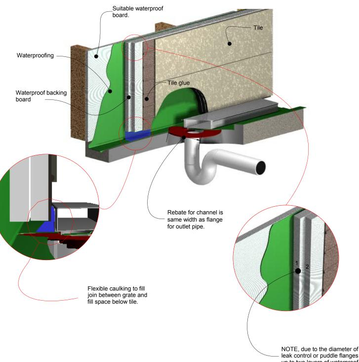
leak control or puddle flanges up to two layers of waterproof backing board or villa board may be needed to pack out wall before tiling.
