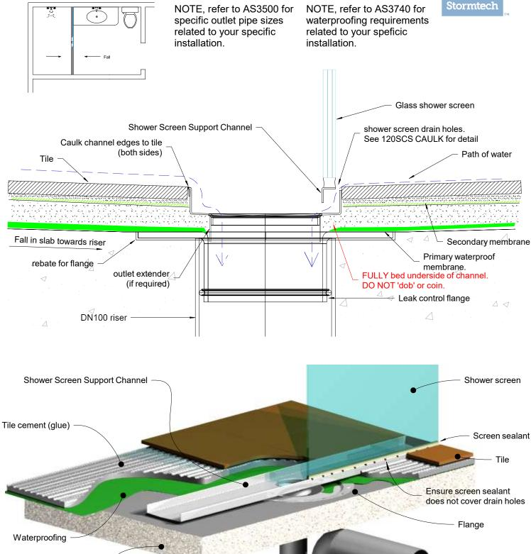
NOTE, this method requires the channel system to be ABOVE and SEPARATE from the WATERPROOFING. NOTE, No grates or tile inserts are shown for clarity.
