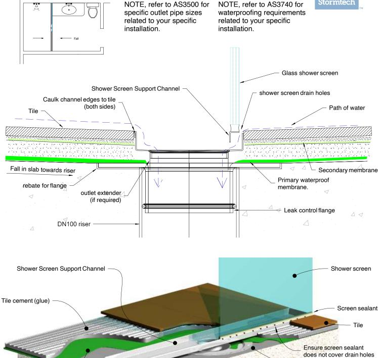
NOTE, this method requires the channel system to be ABOVE and SEPARATE from the WATERPROOFING. NOTE, No grates or tile inserts are shown for clarity.
