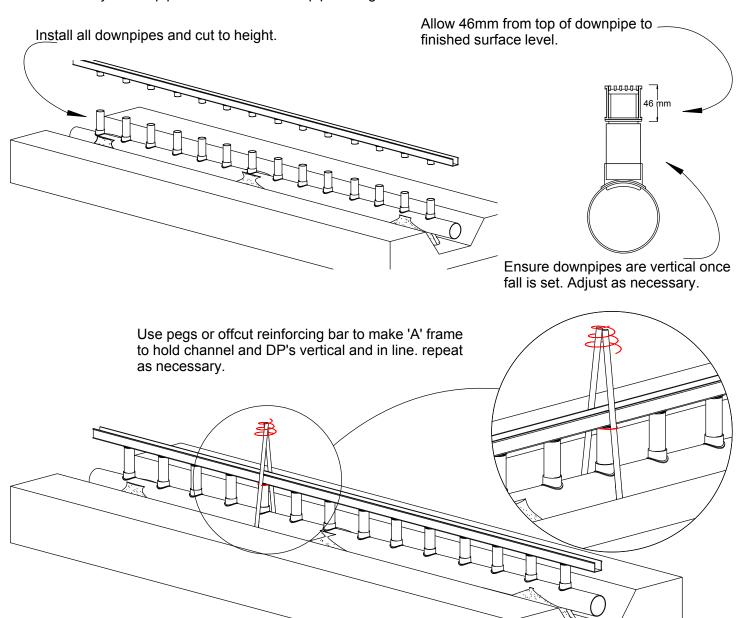
NOTE, When pouring concrete or laying pavers against the channel, ensure the grates are in the channel and protected. If grates are not available use timber form to brace channel. This will ensure the channel remains straight and will also ensure the channel is not squashed and made narrower.
