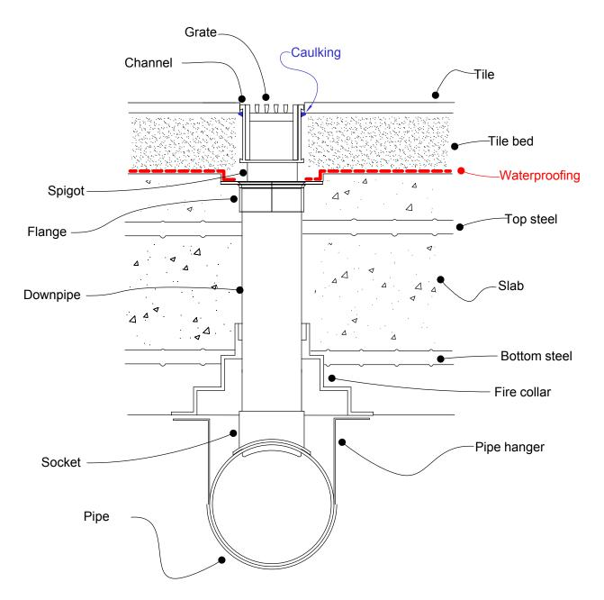
When installing the Special Assembly ensure the pipe is secured, typically to reinforcing or formwork. It is suggested to have the grate and channel in place at time of pour to ensure the Spigots line up with the Downpipes.
