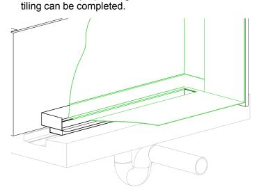
For tiling, ensure the grate is removable and not locked in by tiles.
