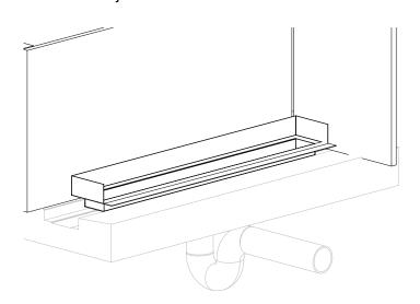
Apply a suiteble waterproofing membrane as per relevant standards and building code. The flanged tray is suitable for use as a waterproofing flange.
