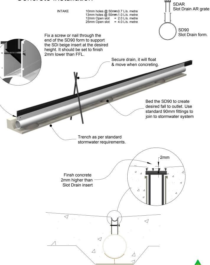
This drawing is the intellectural property of STORMTECH Pty Ltd. Drawings are not to scale. Use dimensions shown.
