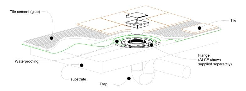
NOTE, this method requires the channel system to be above and separate from the waterproofing
